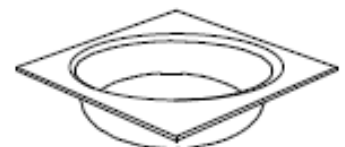
SQUARE DECK AS DEMOLDED FROM AN UNBLOCKED MOLD
