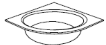
CURVED DECK DEMOLDED FROM A BLOCKED MOLD
