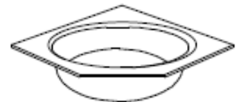
CUT CORNER AS DEMOLDED FROM A BLOCKED MOLD
